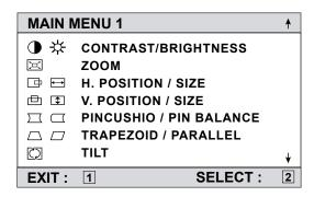
2. To select a setting to be adjusted, press the arrow buttons on the front control panel of your monitor and scroll through the choices. When the desired control is highlighted, press button [2].
